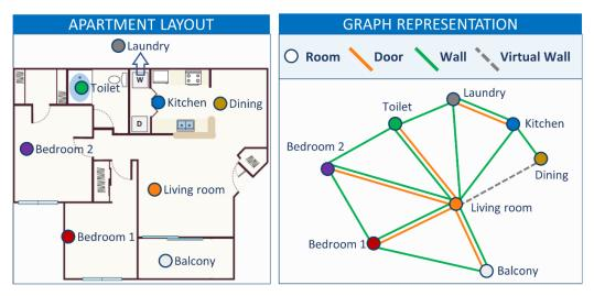
**Figure 2.** Schematic diagram of graph representation for an apartment layout. The lefthand image is an apartment layout, and the righhand image is its graph. Each room is regarded as a node and the relationships between rooms are edges. Three different relationships – door, wall and virtual wal connection – are used for graph construction.
