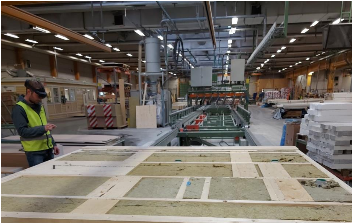
Fig.4 Quality inspection of a timber frame element using HoloLens2
