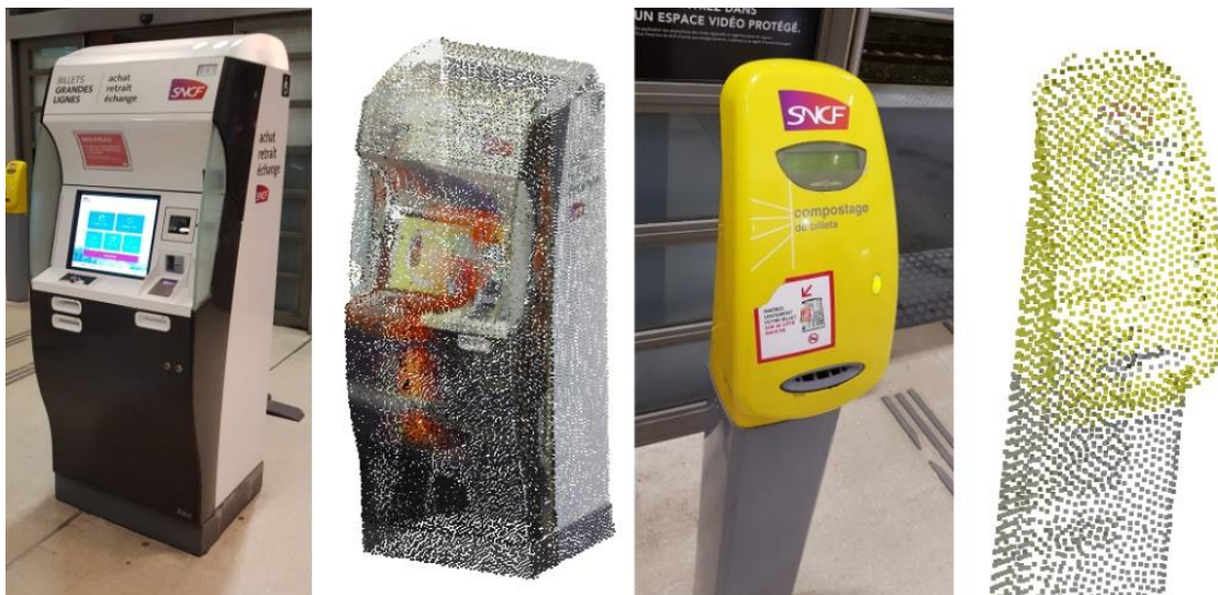
Figure 3. Left: Photograph of a “main line” ticket dispenser and the reference point cloud. Right: A photograph of the second object, a ticket control machine and its reference point cloud.
