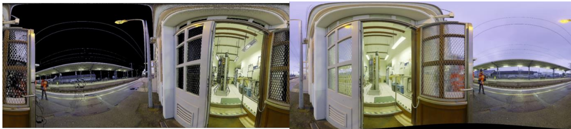
Figure 2. Left: Converted panoramic image from color point cloud. No points have been collected in the sky, as there is no surface. Some artifacts have been caused by people moving through the scene during the scanning process. Right: Actual photo taken by the Lidar scanner. A panoramic photo is periodic, the periodic shift results from the point cloud registration during the acquisition process.
