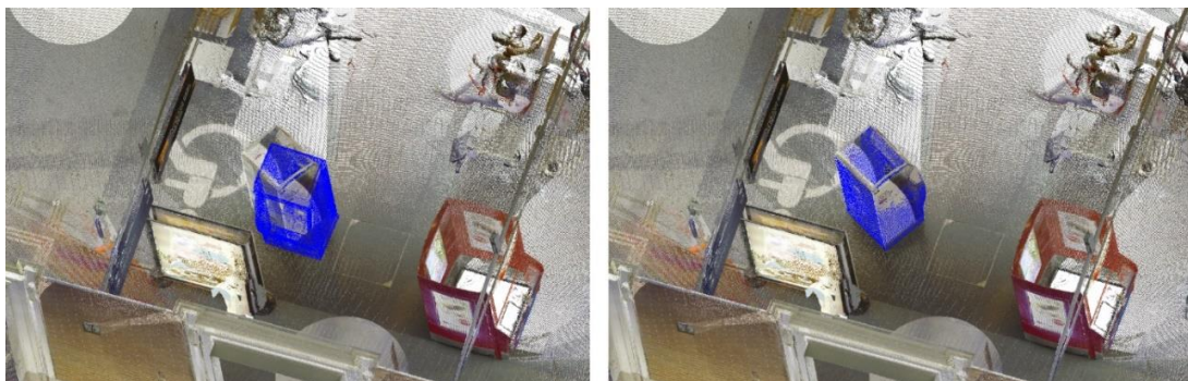
Figure 4. Left: Reference object placed at the estimated 3d position before registration. Right: After registering the reference object is well aligned with the real object.
