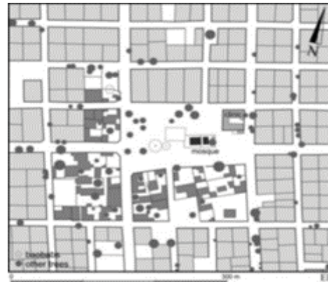
Figure 5: Image after 'smoothing' using Gaussian filter
