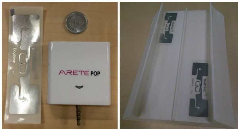
Fig. 94.4 RFID tag and compatible reader and three-dimensional printed model
