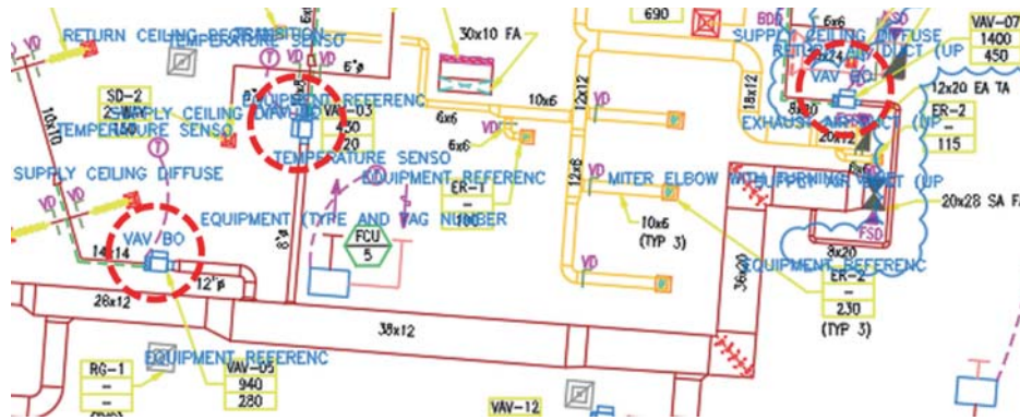
Fig. 60.2 Recognized symbols (VAV BOX highlighted in red dashed circle)
