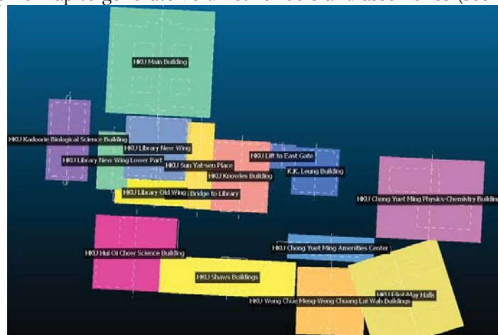
Figure 6: Guide lines identified from building footprints in a sample area of the topographic map
