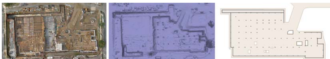
Figure 2: UAV-based photogrammetry for georeferenced point cloud generation and as-is extraction of geometric building model information (from left to right)
