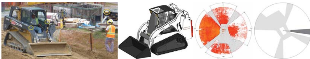
Figure 3: GNSS data evaluation using high-precision differential GPS unit, geometric equipment model (skid steer loader), blind spot diagram of the equipment as used in the field on the 12m visibility blind spot measurement test circle, and geometric blind spot model encountering an obstacle (cast-in place concrete column) in BIM and causing an obstruction to the field-of-view of the equipment operator (from left to right)
