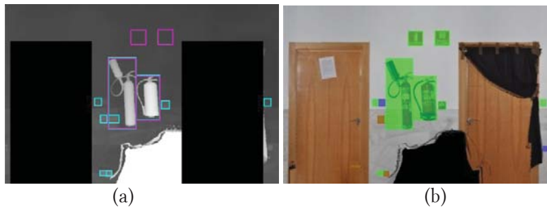
Figure 5: Integration of recognition results. a) Recognized objects by geometry (in cyan) and by colour (in magenta). b) True positives (in green), false positives (in red) and false negatives (in blue).
