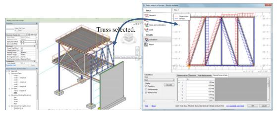
Figure 5. Truss analysis tool.
