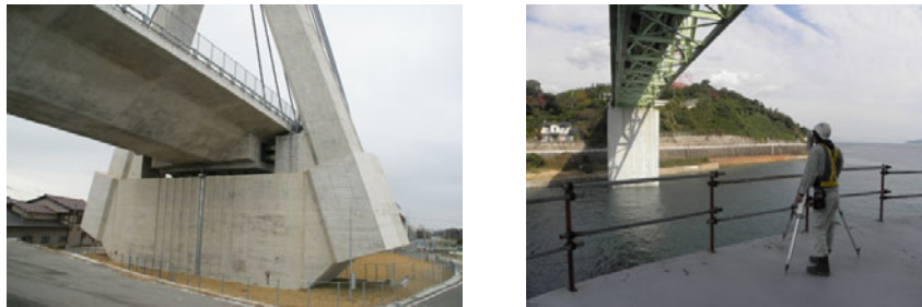
Figure 4. Measurements of a bridge pier using “KUMONOS”.
