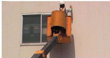
Figure 1. Traditional crack measurement from a lifting cage.
