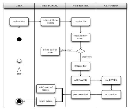
Figure 2: Activity diagram for EAVEK case application.
