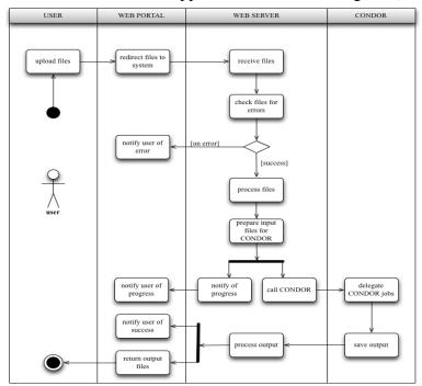
Figure 3: Activity diagram for NANDRAD case application.
