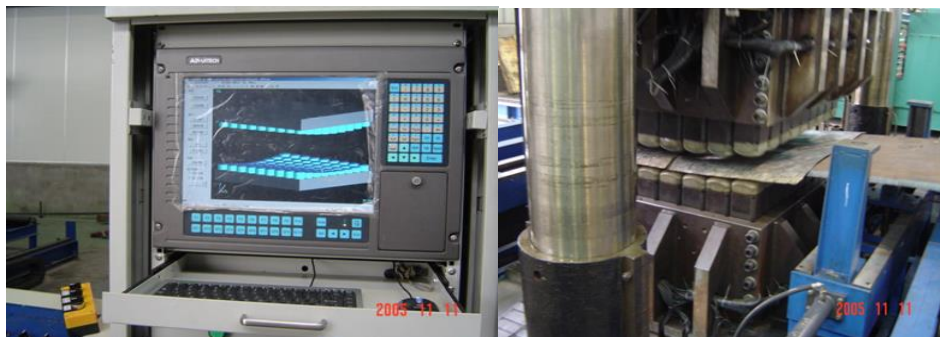
Figure 1: Distorted panel multi-point non-molded forming equipment
