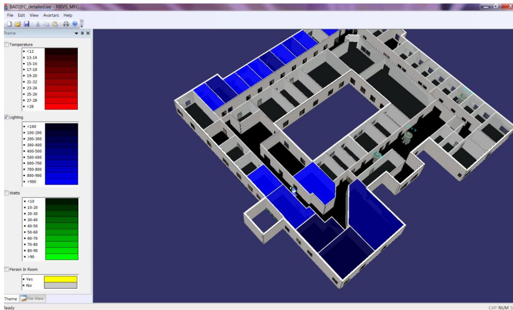
Figure 2: The Snapshot of the RBIVS showing room lighting and people's movement.
