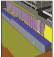
Figure 3: Snapshot 4D model of LPCH Make Ready Utilities tunnel concrete structure construction.
