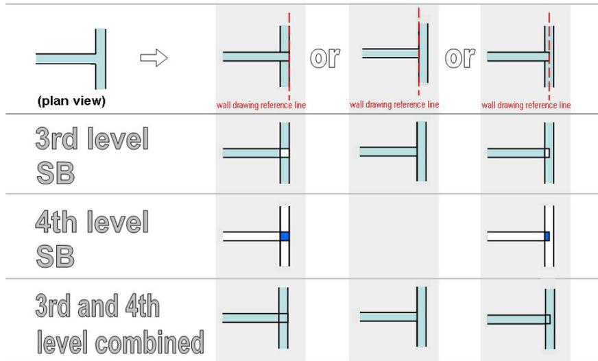
Figure 5: Third (3<sup>rd</sup>) and fourth (4<sup>th</sup>) level space boundaries at wall intersections
