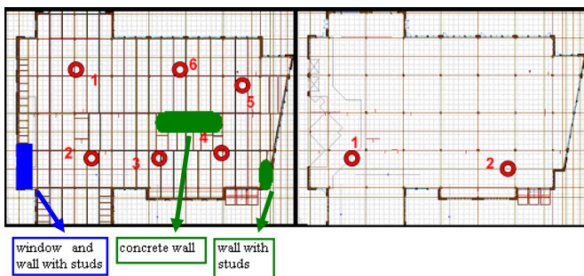
Figure1: Scanner positions, 1.a: AMCW and 1.b: Time-of-flight
