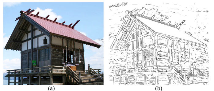
Figure 7. Edge detection result (Meer & Georgescu 2001): (a) Original image (b) Edge detection result
