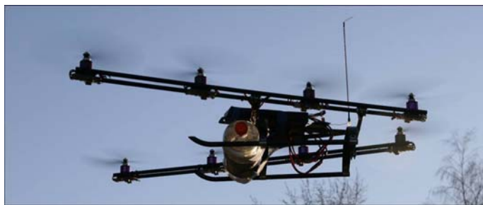
Figure 3. Octocopter developed by DLR, carrying a stereo-photogrammetric camera.
