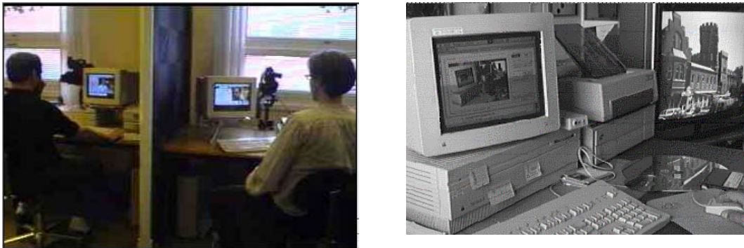
Figure 1: Left; Experimental set-up at KBS-Media Lab, Lund University, 1991, with video communication and screen sharing using Timbuktu from Farallon. Right; A hypermedia workstation developed 1988 at KBS-Media Lab, Lund University with video display of images and films stored on video disk integrated with the hypertext based program HyperCard from Apple computer. From (Christiansson 2001b).
