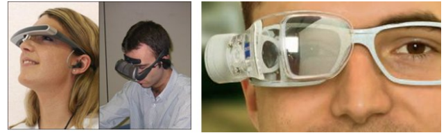
Figure 4. Video-through and see-through visualization devices.
