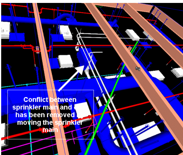
Figure 7. The picture at the top shows a clash or conflict between a supply duct and a sprinkler main pipe, highlighted in red. The picture at the bottom shows that the clash was resolved by moving the sprinkler main to the right of the duct. These clashes were first identified by using the NavisWorks' clash detection program and resolved in a subsequent clash resolution session. Image courtesy, DPR Construction, Inc., CA, USA.
