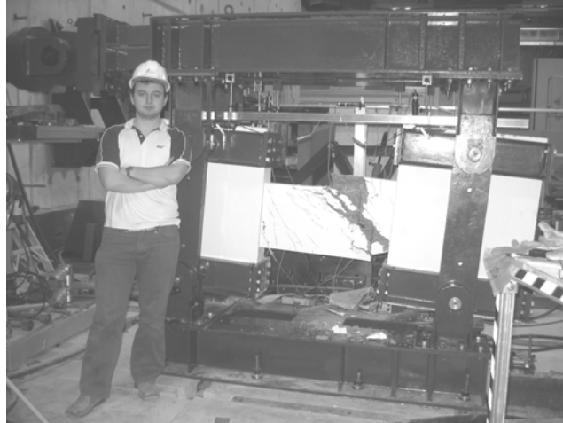
Figure 4: Test Rig with Tested Specimen
