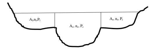
Figure 2: Division of the Flooded Natural Cross Section into Discrete Elements
