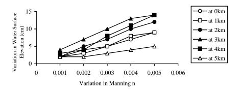
Figure 4: Effect of Manning Roughness on the Predicted Water Surface Elevation Along the Linggi River
