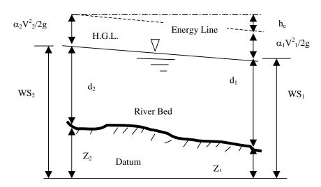
Figure 1: Profile of Natural River Reach with Two Stations
