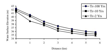
Figure 5: Predicted Water Surface Elevation for the Linggi River
