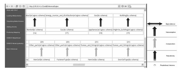
Figure 1: Partial representation of OSIECS model showing subsumption and conjunction mappings between the eCognos and the *bcBuildingDefinitions*
