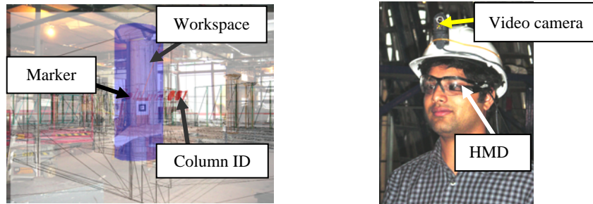
(a) Augmentation of the column as seen by the superintendent (b) Construction superintendent equipped with AR devices
