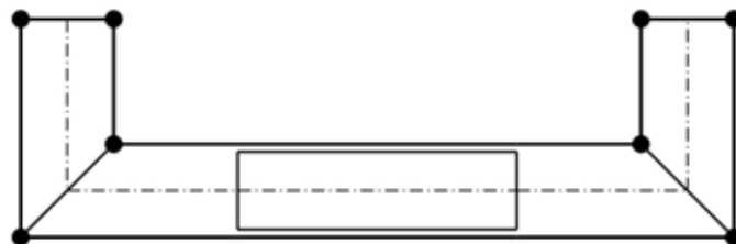
Figure 6: Construction model and system model of a coign identified in a ground plan (G1).
