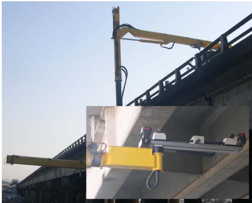
Figure 10: Remote Control Inspection Robot for Bridge
