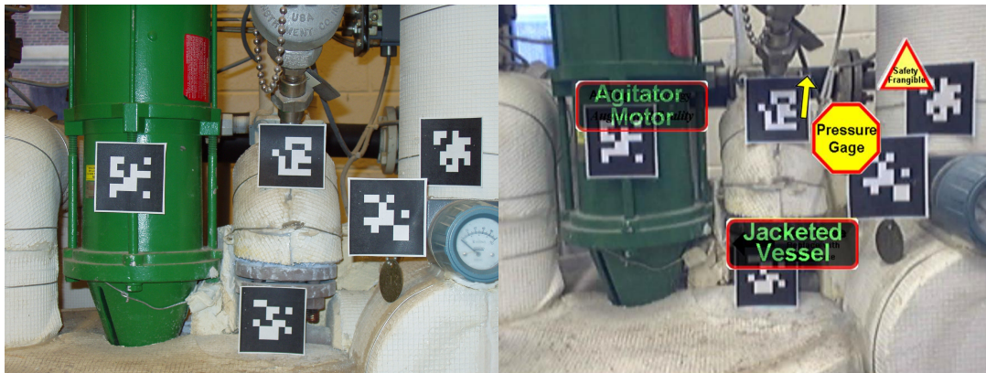
Figure 3. Scene of Markers Arrangement on Equipment (Left) and Augmented Reality Scene with Virtual Tags Overlaid onto the Real Counterparts (Right)
