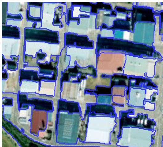
Fig.2 Building contour extracted from aerial photo by pattern recognition (eCognition, Definiens Inc.)
