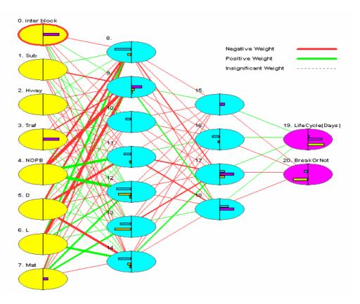
Figure 3: Artificial neural network (ANN) model of the risk factors for failure
