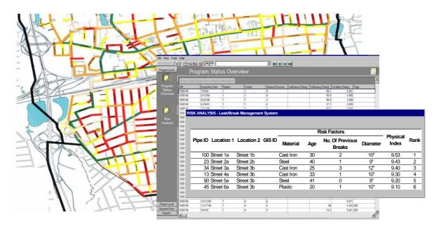
Figure 1: GIS-based management system for water distribution networks (graphical interface)
