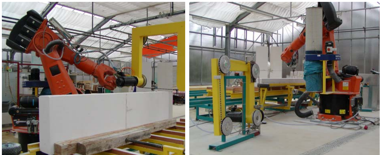
Figure 7: Prototype of a robot cell (left with a wire saw, right with a milling spindle).
