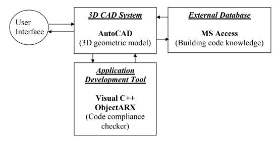
Figure 2. Architecture of the Automated Code Compliance Checking System
