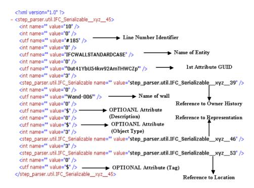
Figure 7: The XML Serialization of an IFCWALLSTANDARDCASE to an XML file
