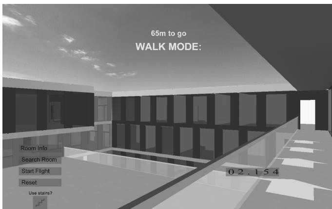
Figure 2. A sample guidance system – here shown as VRML application – based on the graph derived from the computer science building of Universität Stuttgart.
