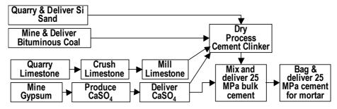
Figure 4 Process map for cement mortar
