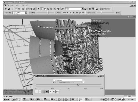
Fig. 6. 4D Modeler and TimeController. Both views display the same date, 2002-04-22.
