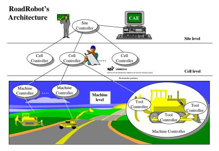
Figure 2. Architecture of RoadRobot project - Logical levels
