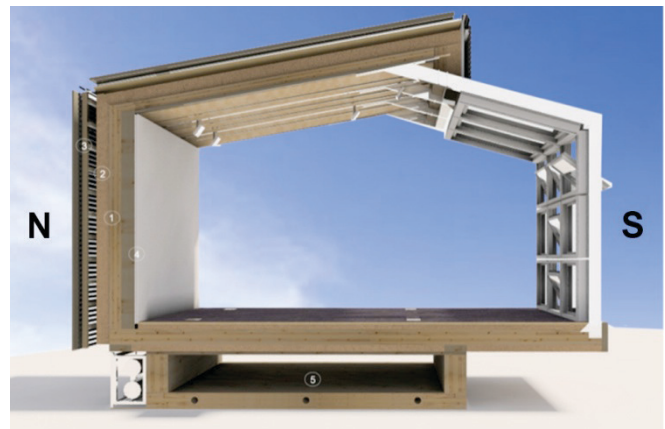
Figure 4: Two extreme systems of sustainability were combined: passive/north (left) and active/south (right).
