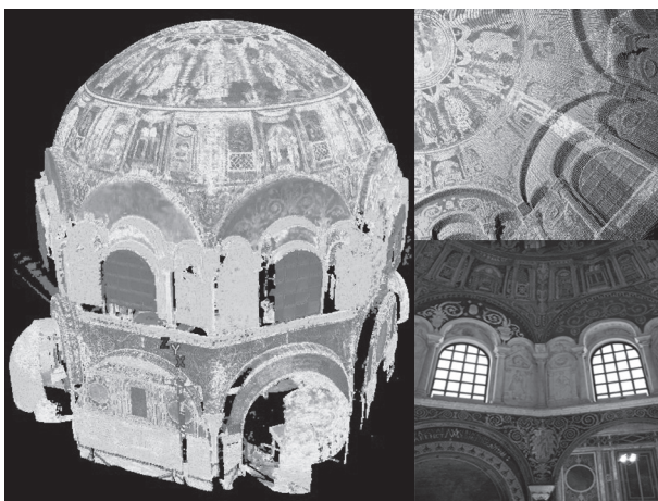
Fig. 3. Phase-based 3d scanner of mosaics of Battistero Neoniano in Ravenna.
