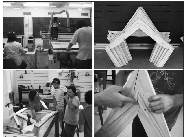
Figure 2. CNC fabrication of 890 differentiated components
