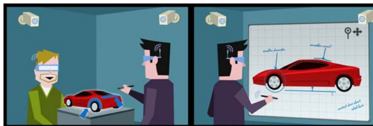
Figure 2: Collaborative car design review scenario combining large and head mounted displays (conceptual sketches)
