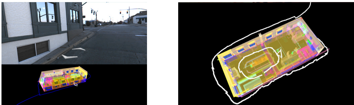
Fig. 1: Prototype view showing map, paths, camera position, translation arrows, and scene view (left). Model, seen from the top, showing 2 camera paths and virtual camera frustum (right).
