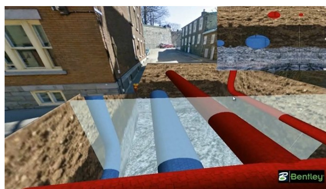
Fig. 2: Virtual excavation for subsurface utilities as shown in (Côté, 2011b).
