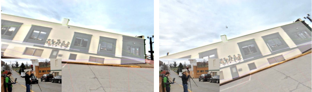
Fig. 8: Two frames extracted from the camera rotation experiment. Tracking produced no augmentation jitter, but a small amount drift accumulates over time (see rightmost part of right image).
