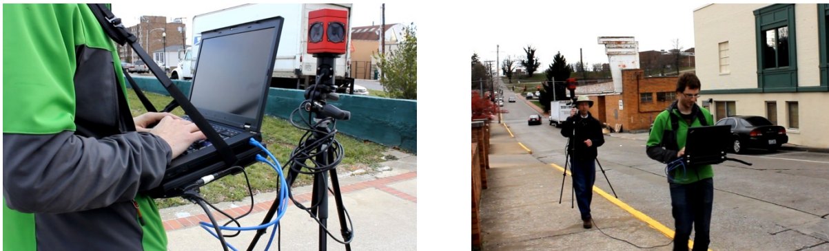
Fig. 7: Setup for carrying the computers and camera on site.
