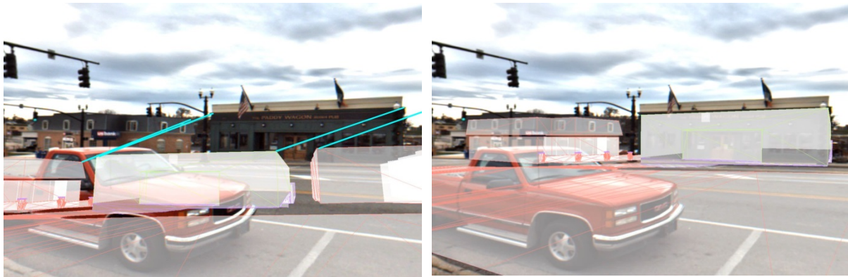
Fig. 2: Initialization process. Left: Correspondences selected by user. Right: The pose calculated from those correspondences is used to align the panorama and the tracking model.
