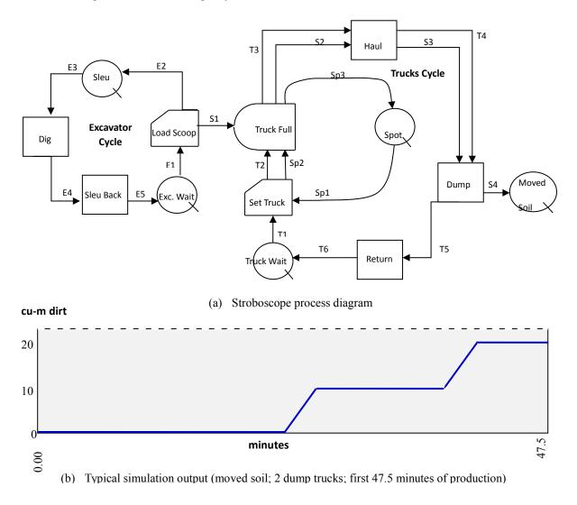
Fig. 2: Stroboscope model of an earthmoving operation (see Martinez (1996)).
