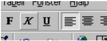
Figure 5.4 Detail from a Windows user interface. The function for justifying text to the left is selected and the pointer (not visible in the figure) is held over the tool for italic text (the letter K stands for kursiv, italic in Swedish). Note how shadow effects create the impression of buttons that are pressed or ready to be pressed and that the light source seems to be situated in the upper left corner of the picture.
