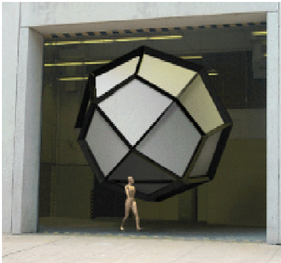
Fig 3 - How a 24-facet immersive display structure might be located within a high ceiling room. The entrance shown is about 6 meters wide.
