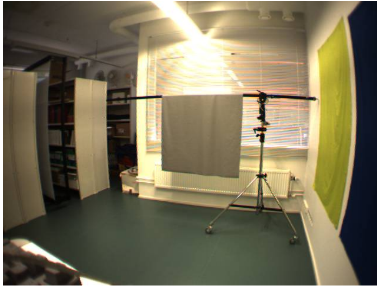
FIG 5: Example of wide angle lens effect to the resultant picture.
