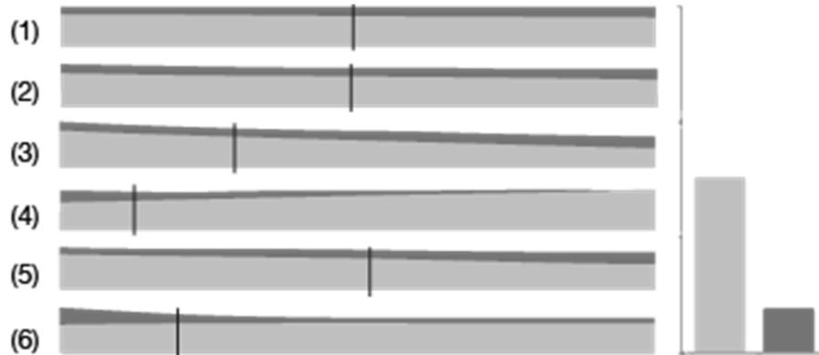
**Figure 1. The output of the model shows the current selected parameters with their specific performance graph and the calculated heating (light grey) and cooling (dark grey) demands. It also displays how the parameters have to be changed to obtain a more effective solution.**
