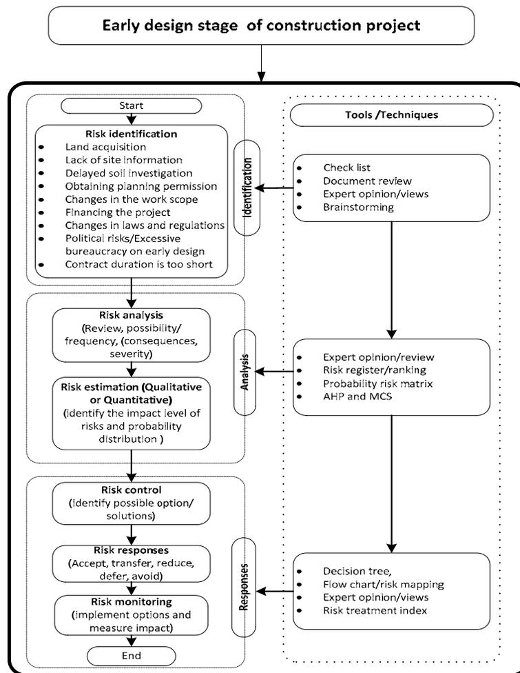
**Figure 1. Framework of CRMM at the design stage of a construction project Information Flow Diagram.** The specification of the framework is presented in the form of information flow diagram. The information flow diagram of the CRMM is shown in Figure 1. The diagram contains a total of nine steps that need
